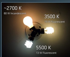
IMAGE 13. COLOR TEMPERATURE EXAMPLE. THREE BULBS ARE USED IN TWO CATEGORIES (INCANDESCENT AND FLUORESCENT LAMP) AND DIFFERENT COLOR TEMPERATURE. LOW TEMPERATURE SOURCES TEND TO BE WEIGHTED TOWARDS THE RED END OF THE SPECTRUM, WHILE HIGH TEMPERATURE SOURCES ARE TOWARDS THE BLUE END OF THE SPECTRUM.
